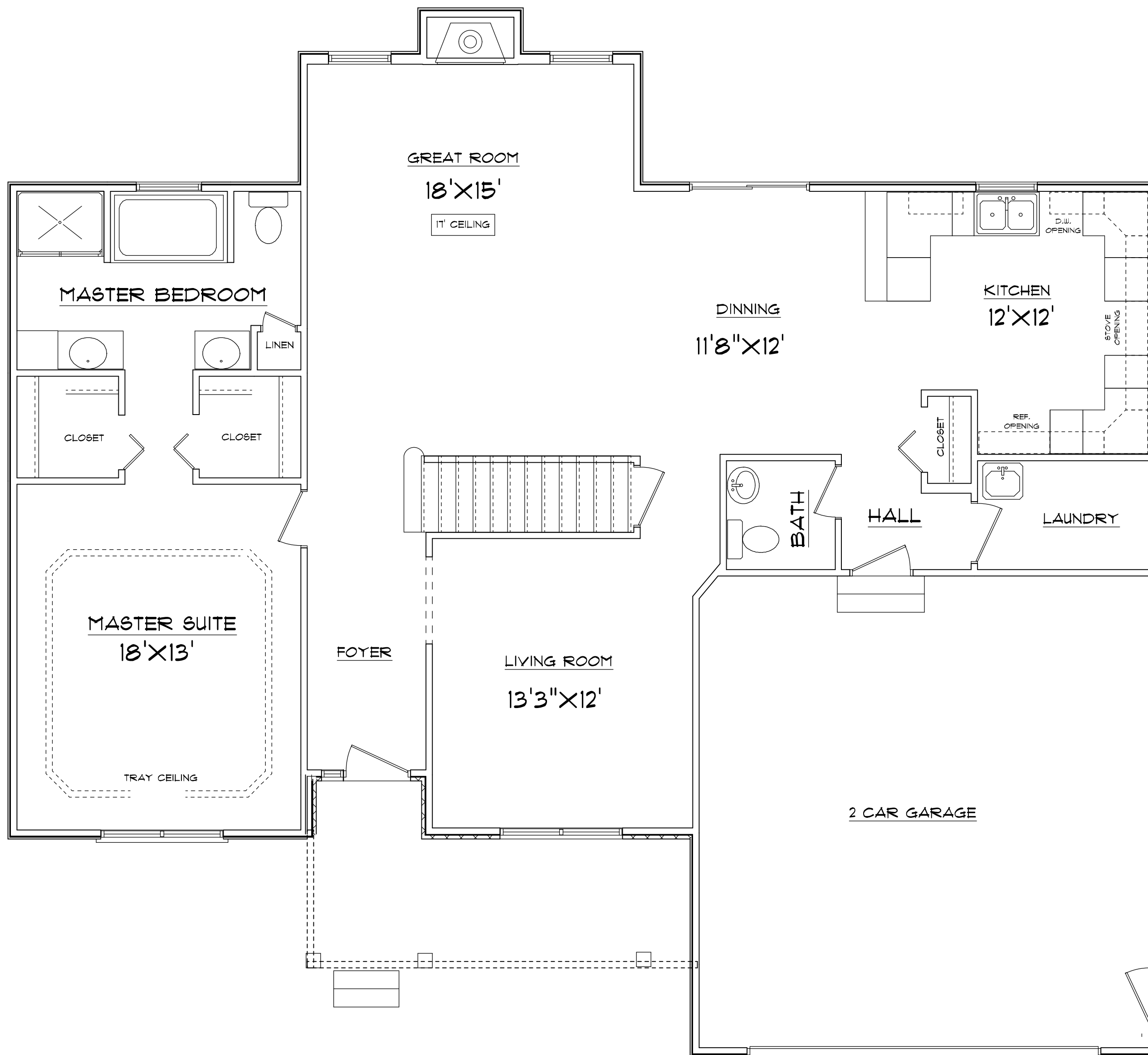
1ST FLOOR LAYOUT SCALE: 1/4" = 1'-0"
